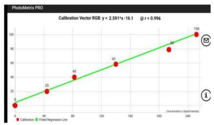
Figure 8 Calibration graph obtained from PhotoMetrix Application
